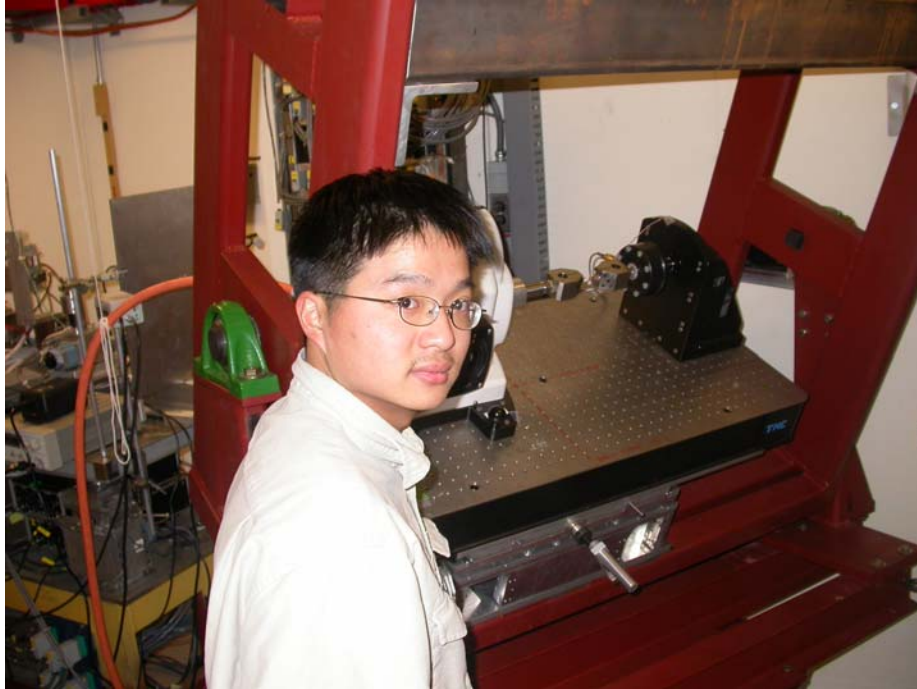
Master of Engineering student Phil Wu stands in front of the load-frame inside the A2 x-ray station. The “jaws” in the center of the tilted load-frame hold a copper specimen that is stretched during the x-ray measurement. [Photo: Matt Miller]
