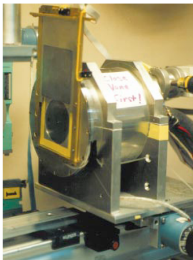
Photograph of the CCD detector in place at the CHESS A1 station. A protective metal screen (shown open at left) protects the phosphor when not collecting data.
