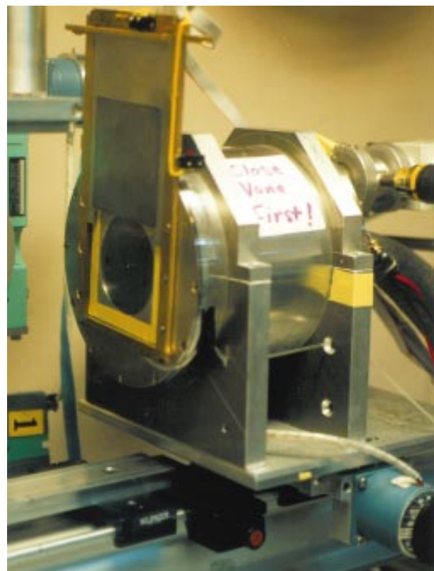
Photograph of the CCD detector in place at the CHESS A1 station. A protective metal screen (shown open at left) protects the phosphor when not collecting data.
