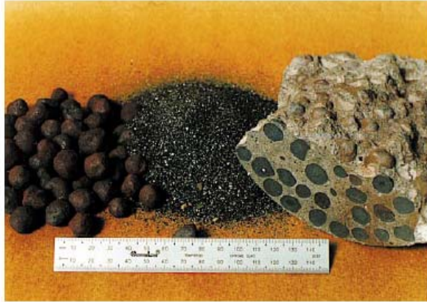
The photo shows a cut away section from an early test sample of heavy concrete. The mix was designed and tested at Cornell. The fine ore and coarse pellets are highly enriched with iron and replace sand and gravel to improve neutron shielding. The pellets are an inexpensive substitute (made for the production of steel) for high-grade, natural iron ore that is commonly used to produce this type of concrete.
