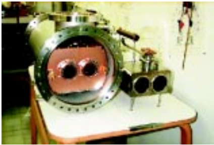
Prototype section of a proposed dual-bore superconducting storage ring.
