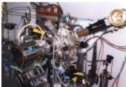
Figure 1: The ultra-high vacuum thin film growth chamber set up in the A-2 hutch. The two-theta arm with detector is at the right, and a Si(Li) detector for energy analysis of X-ray fluorescence from the sample is in the left foreground.
