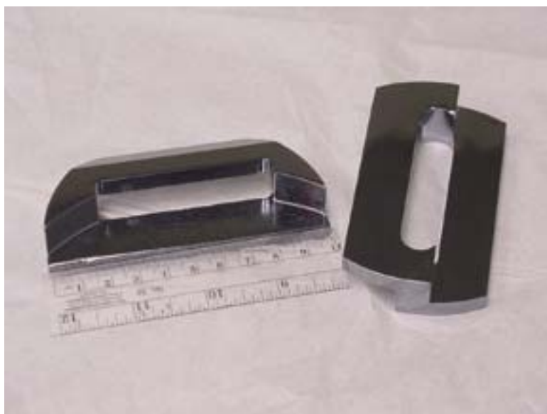
Fig. 4 Silicon channel cut crystals for the 4-bounce monochromator provide narrow bandwidth and high flux. These crystals utilize (111) reflections; the left (right) crystals operate between 7 and 10 (12 and 19)KeV. High order reflections are used for higher energy resolution.
