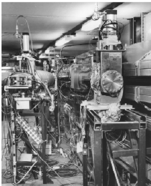
Fig 4: First CHESS A (left) and B (right) beamlines as photographed by C. Hadley Smith on 6/29/79. The A-line beamline ends in the Hartman split ion chamber for beam position measurement. The inner plates can be seen through the transparent Kapton window. Just upstream of it is the several meter long acoustic delay line with 7 sections. The seven sections were made of large stainless steel mixing bowls with slots cut in the orbit plane to let SR through but to slow any inrush of air should a window fail. On the right B-line beamline, the acoustic delay line is not yet attached as it was still coming off the production line. Signals were run back to the CHESS control room through the trenches from patch panels we scrounged up from the CESR group of C. O. Brown and Mike Ray.
