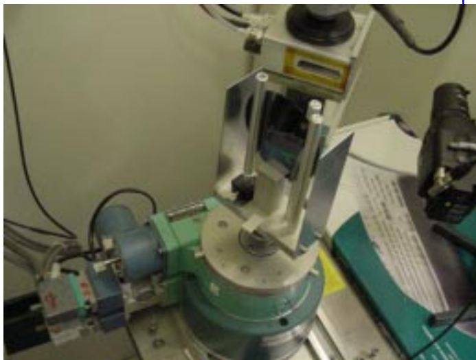
Fig 5: The simple three-rod bender mechanism used to curve an ultrathin silicon crystal wafer. The incident broad bandwidth x-ray beam from the main multilayer monochromator comes in from the left. Approximately 1% of the beam is diverted through the ion chamber (top) into G2 hutch.
