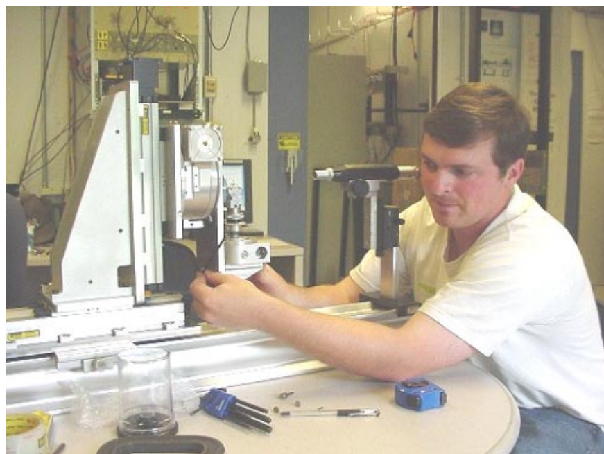
Fig 2: Sterling Cornaby aligning the new G1 monochromator/GISAXS goniometer.
