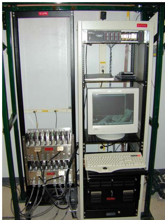
Fig 1: G-line motion control system. All necessary hardware is located inside the hutch and controlled via the computer network.
