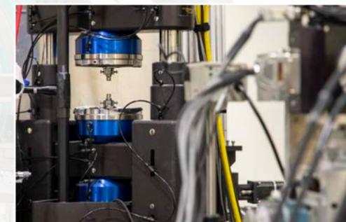
The Forming and Shaping Technology (FAST) beamline is designed to study the processing and performance of structural materials with a focus on in-situ experiments. Users are able to perform a wide-range of high-energy X-ray diffraction and imaging measurements including near-field and far-field high-energy X-ray diffraction microscopy, powder diffraction, and micro-computed tomography.
