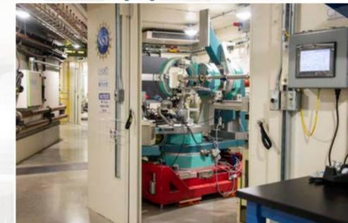
The QM2 beamline (at CHESS endstation 4B) is dedicated to high throughput characterization of quantum materials in reciprocal space ("Q-space"). The beamline is optimized for both resonant scattering studies and high-dynamic range mapping with high energy photons. The ability to switch easily between these configurations for each sample under study enables comprehensive measurements, performed quickly.
