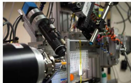
These beamlines are devoted to monitoring the structure of the building blocks of life at the molecular level under high pressure, e.g. found at the bottom of the ocean, an important regime not previously accessible to biologists. The macromolecular crystallography (MX) beamline determines the atomic structure of macromolecules in a diamond anvil cell at pressures up to 400MPa. The high-pressure small angle scattering beamline (SAXS) determines the shape at pressures up to 700 MPa.
