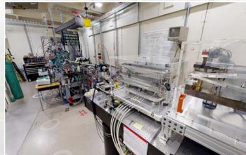
PIPOXS provides high intensity x-ray beams for use in various X-ray spectroscopic techniques—including X-ray absorption, X-ray emission, and resonant inelastic X-ray scattering—over an energy range of 3.5 – 60 keV. The large PIPOXS hutch allows for a wide variety of spectrometers and sample environments to be accommodated.
