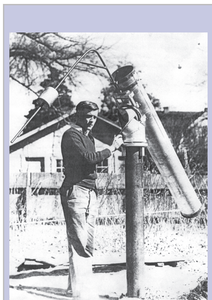
Fig 3: The photo shows Paul Hartman as a young man after building this telescope. Paul told Ken Finkelstein (CHESS staff scientist) that he built it while an undergraduate at the University of Nevada. Paul fabricated all the components himself including the 8" parabolic mirror, the Springfield mount and the gear system. This style of mounting allows one to sit on a stool and look through the lens without changing orientation while the scope is pointed anywhere in the sky. Paul cast the entire gear assembly and machined the teeth on the two meshing gear wheels. He also ground a number of lenses used with the telescope.
