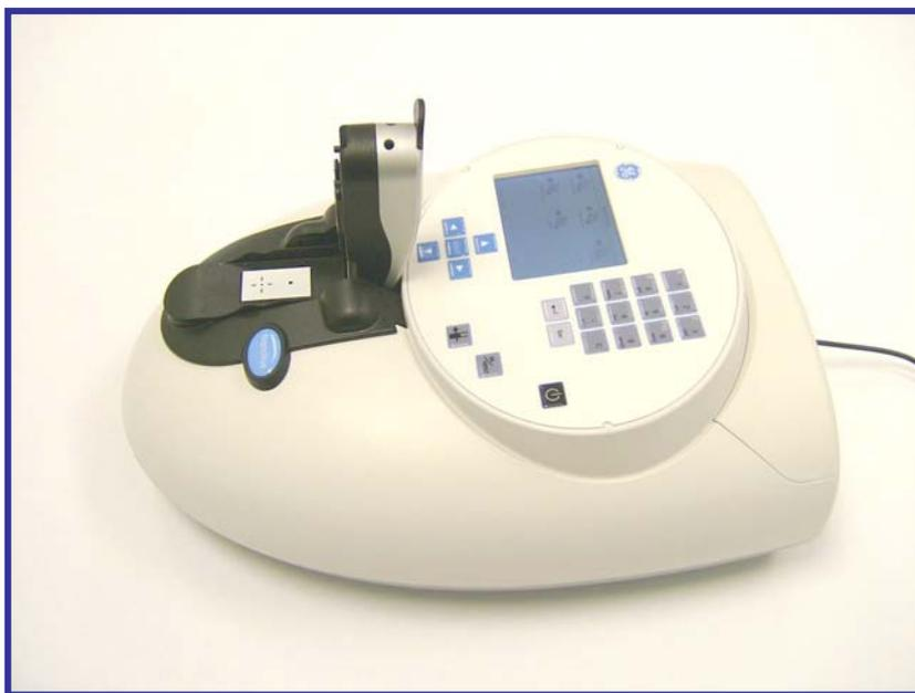
**Figure 1: NanoVue Spectrophotometer**
