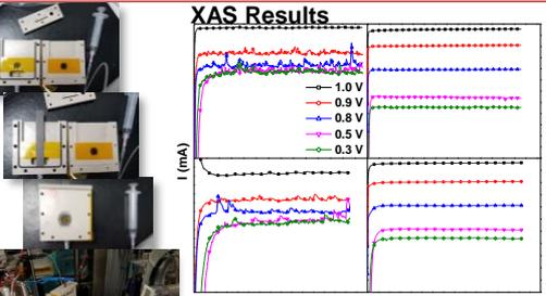
Fig 8: N<sub>2</sub> and O<sub>2</sub> chronoamperometries of PtNi-NWs. 1<sup>st</sup> row plots while Ni edge and 2<sup>nd</sup> row while Pt edge. 1<sup>st</sup> column with N<sub>2</sub> purge and 2<sup>nd</sup> column with air purge.
