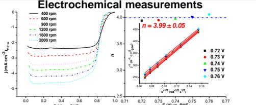
Fig 5: Koutecky-Levich plots of the lab-made PtNi-NWs. ΔE<sub>1/2</sub> = 5 mV
