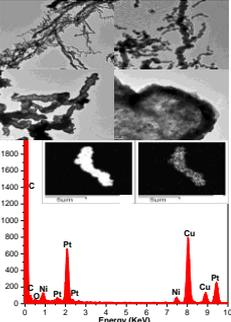
Fig 2: TEM images and EDS mapping of PtNi-NWs.
