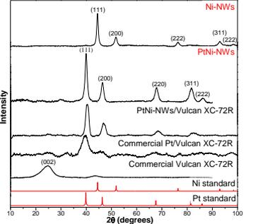
Fig 3: XRD patterns for Ni-NWs and PtNi-NWs.
