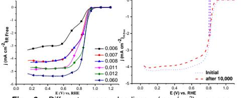
Fig 6: Different mass loadings (mg<sub>Pt</sub>/cm<sup>2</sup>) oxygen polarization curves and durability experiments of PtNi-NWs.
