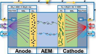
Fig 1: Representation of a hydrogen-based AEMFC with the main species being generated in the cell.
