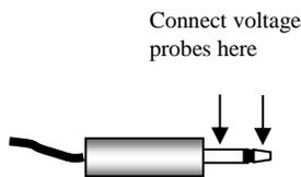
Figure 5 – Photodiode set-up, plug end
