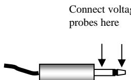
Figure 5 – Photodiode set-up, plug end
