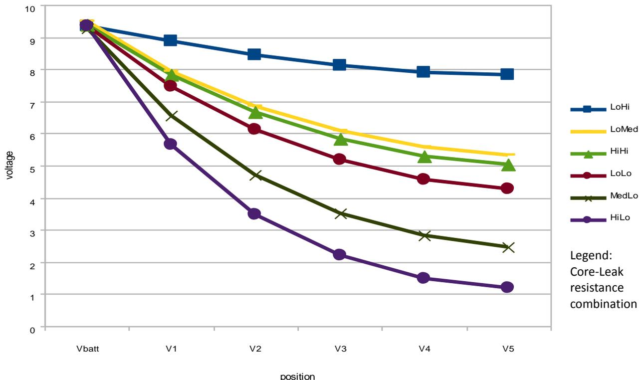
**Figure 5: Voltage Divider Data for Different Resistor Combinations. The core resistance is listed first and the leak resistance is listed second.**
