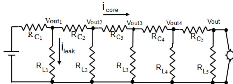
**Figure 3.** Circuit model for signal losses along a cable
