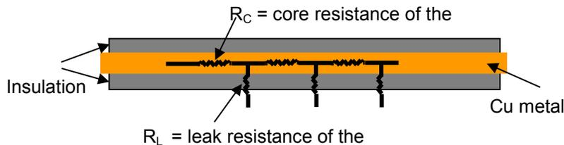
**Figure 2.** Cross-section of an insulated metal wire.
