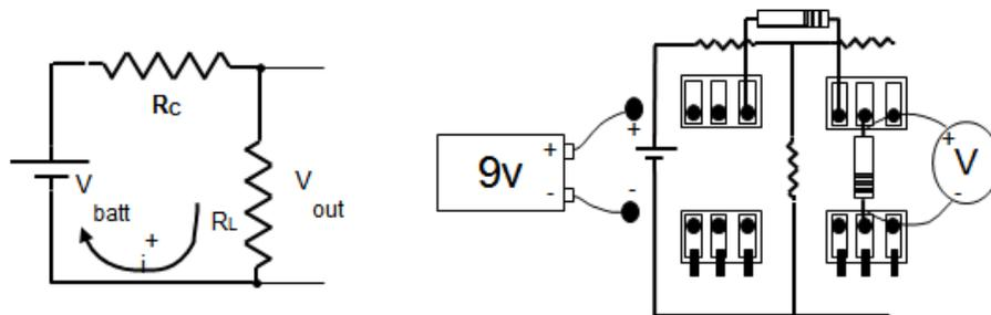
**Figure 4.** Voltage divider circuit and project board wiring diagram.
