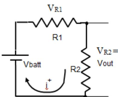
**Figure 1.** A simple voltage divider. Positive current ( $i$ ) flows from the positive pole of the battery through two resistors in series to the negative pole of the battery.
