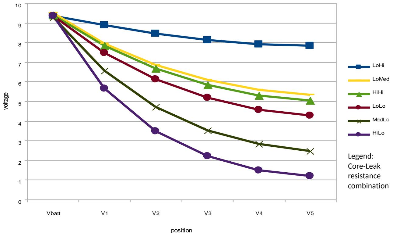
**Figure 5: Voltage Divider Data for Different Resistor Combinations. The core resistance is listed first and the leak resistance is listed second.**
