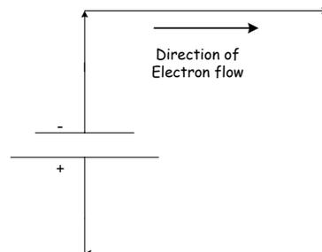
In a very real way, electrons are attracted to the positive terminal and repelled by the negative terminal. The negative electrons are releasing their energy as they move through the circuit, like a compressed coiled spring does when it is released. Any material that connects the terminals and allows the flow of charge is called a "conductor." The circuit diagram here is called a schematic diagram, or
