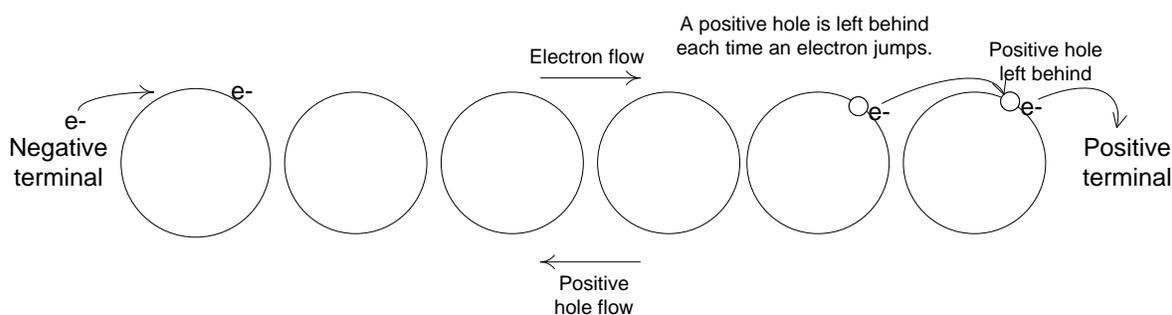
This diagram shows part of a current flowing through a series of atoms in a conductor. Your mission is to complete the diagram, showing how electrons and positive holes move through the conductor. The units of current will be discussed after you have done part of the lab.
