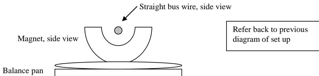
Keeping the length and position of the wire constant, adjust the current in 0.5A increments. Take measurements of the change in the apparent mass of the magnets for each current tested. Use this apparent change in mass to determine the force on the wire. Record your results in the data table on the student data sheet.
