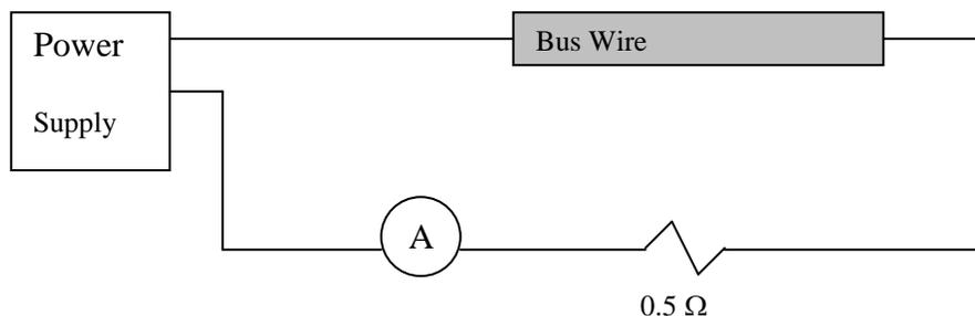
**Activity III:** Changing the length of the wire between the Fahnestock clips is awkward and works best if two people work together. One person adjusts the clamps holding the dowels to the crossbar while the other person simultaneously squeezes the Fahnestock clips to allow the wire to slide and adjust.
