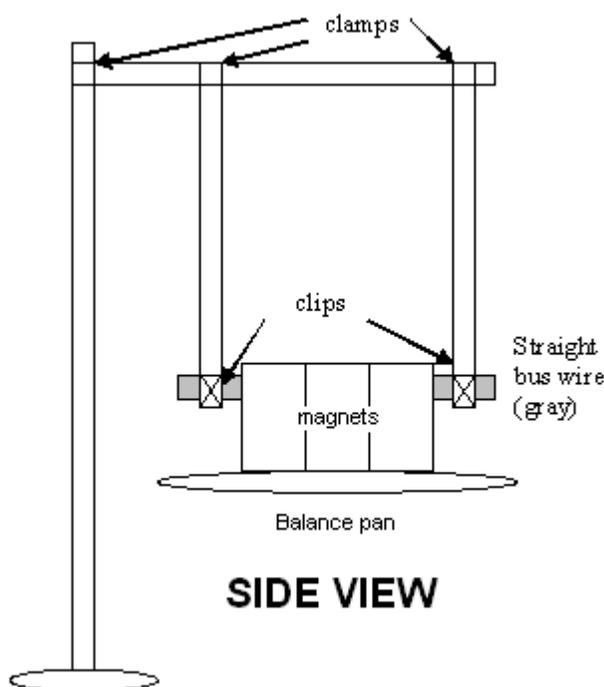
**Activity I: How does the direction of the magnetic force on a current-carrying wire relate to the direction of the magnetic field and the direction of the electrical current?**
