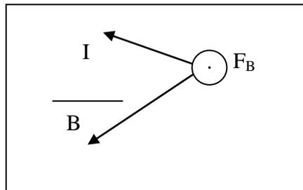
Overhead view, looking down on the plane defined by I and B. In this two-dimensional drawing, the force vector comes out of the page and is indicated by a circle with a dot in the center (as if you are seeing the arrowhead coming towards you). If the I and B vectors were reversed in order, the force vector would be going into the page and would be represented by a circle with an x inside, as if you were seeing the arrow tail as it moved away from you.
