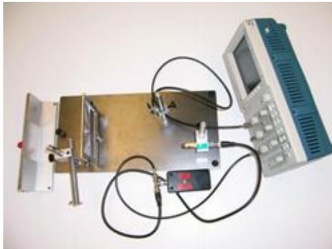
Figure T-2: The oscilloscope and pulse generator w/ the beam-splitter, Fresnel lens, photo detector and laser mounted on the base plate. (Note: The system works better with the beam-splitter on the other side of the Fresnel lens as described in the lab.)
