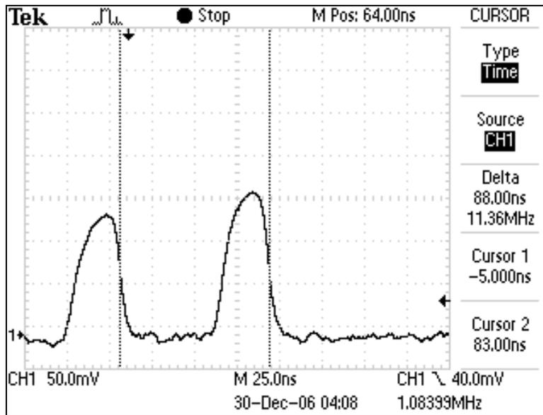
Figure 3: Sample Oscilloscope Screen with far mirror 13.1 meters from beam-splitter. (Note the positions of the vertical cursors and the display of their positions on the screen.)
