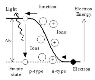
Figure 2. Operation of an LED
