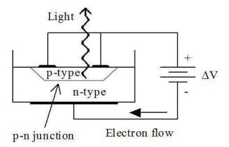
Figure 1. A light-emitting diode (LED).
